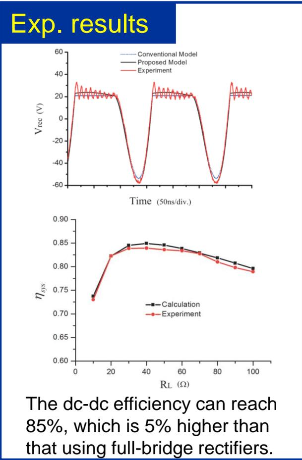
The dc-dc efficiency can reach 85%, which is 5% higher than that using full-bridge rectifiers.
