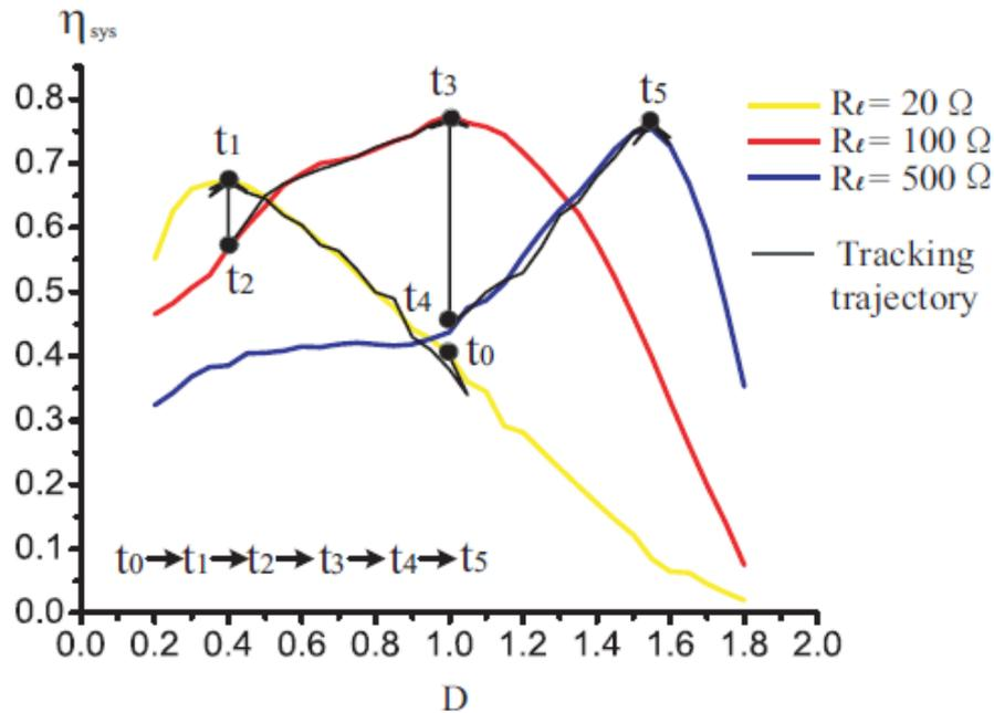
The system can track the maximum efficiency under load variation.
