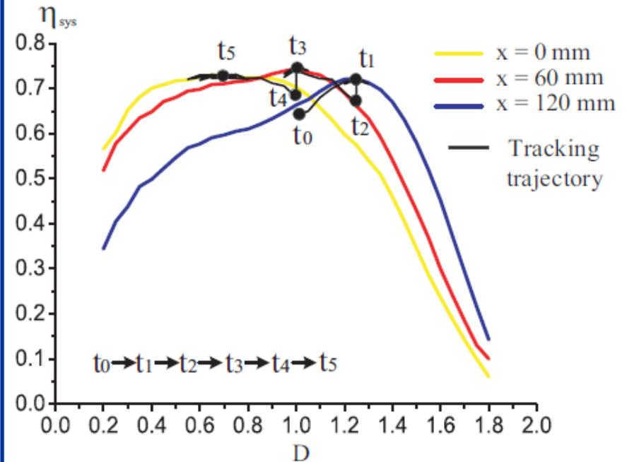
The system can track the maximum efficiency under position variation.
