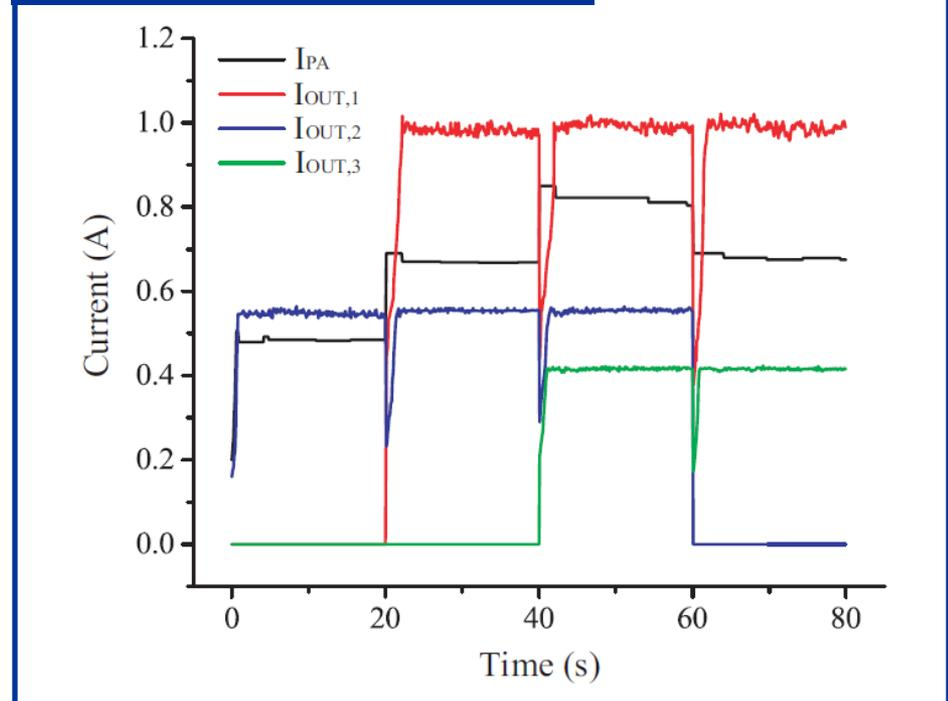
The system can provide a constant output voltage for each receiver with optimized efficiency (**>63%**).
