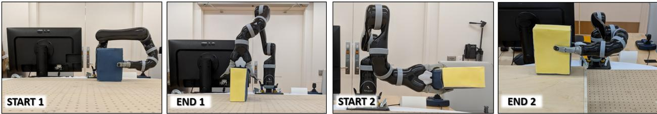
Fig. 2. Example tasks. Start and End 1 depict the starting and ending pose of feature set  $[0, 0, 0, 1, 0, 1]$  which models pure rotations: the user picks up the object, rotates it, and places it in the same location. Start and End 2 depict the starting and ending pose of feature set  $[1, 1, 1, 1, 1, 1]$  which models rotation about and translation through all three axes.
