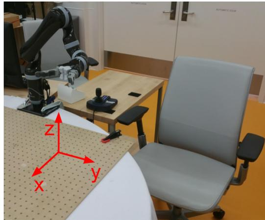
Fig. 1. Mico arm, 3-axis joystick, and world frame ( $x$ -,  $y$ -,  $z$ -axes).
